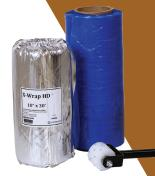
X-Wrap HD (formerly IRO HD - Impact Resistant Outerwrap-Heavy Duty) is designed to protect field joint coatings and mainline coatings from abrasion and mechanical damage. X-Wrap HD consists of pre-impregnated woven glass fabric and water activated resin. This product is designed for use during tunneling, horizontal directional drilling (HDD) and bores. X-Wrap HD supersedes IRO HD products and should be substituted for all future use.
